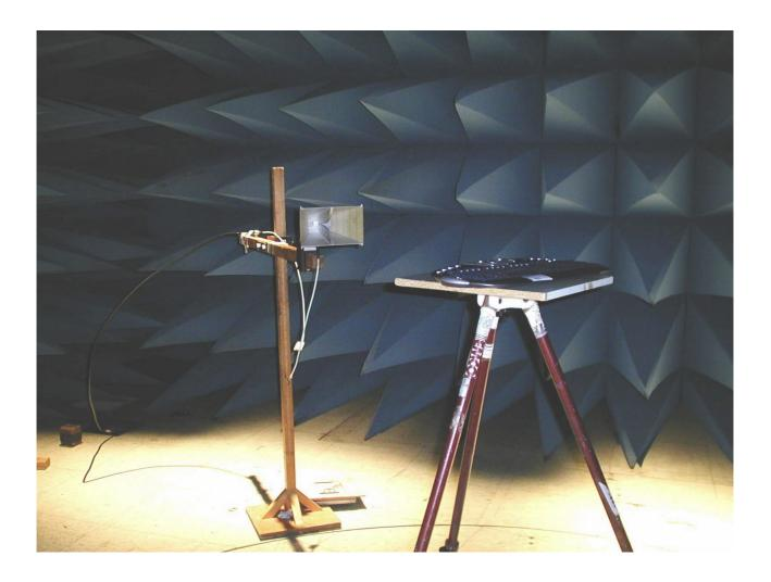
Test set-up for RF conducted measurements.
