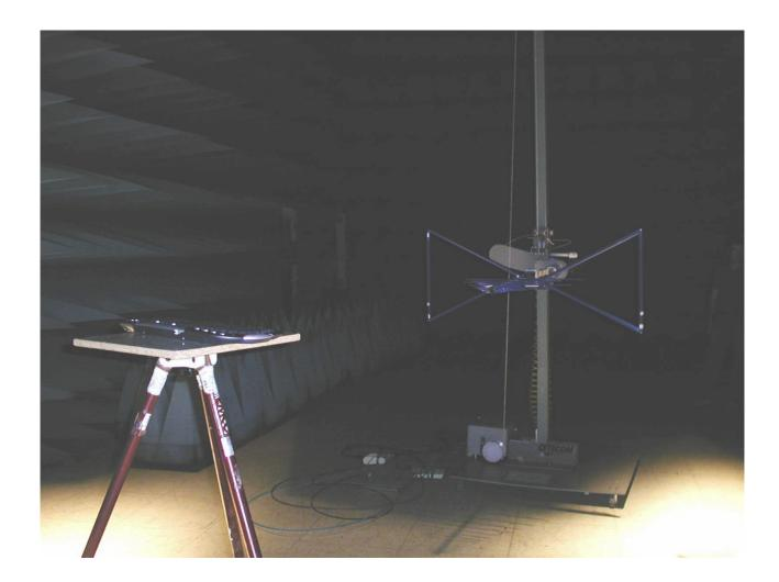
Test set-up for radiated measurements above 1 GHz.
