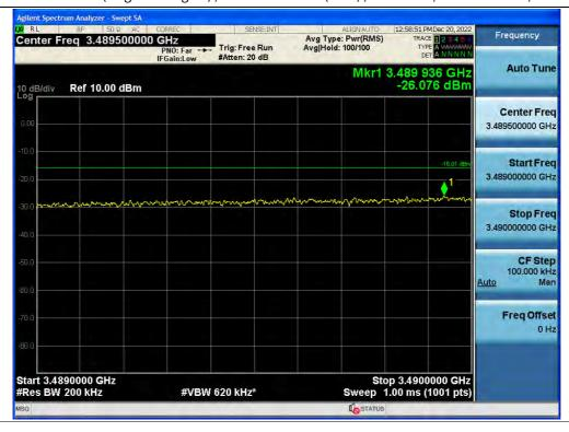
+3 dB above Out-of-band (single test signal) / 3.45 GHz Service(Ant2) / Downlink / 5G NR 20 MHz / Middle / Upper
