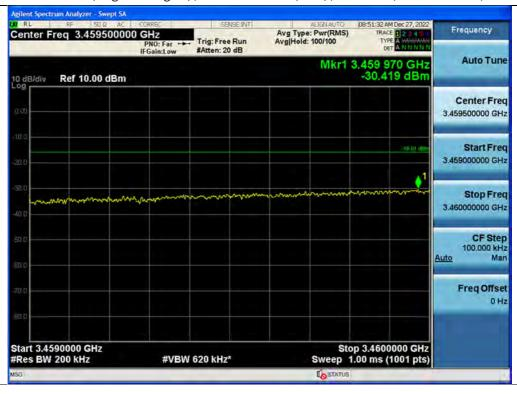
+3 dB above Out-of-band (single test signal) / 3.45 GHz Service(Ant1) / Downlink / 5G NR 80 MHz / Middle / Upper
