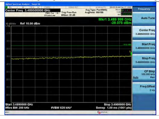
+3 dB above Out-of-band (single test signal) / 3.45 GHz Service(Ant1) / Downlink / 5G NR 60 MHz / High / Upper
