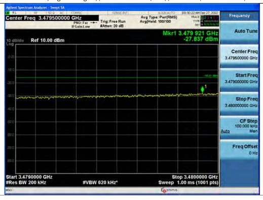
+3 dB above Out-of-band (single test signal) / 3.45 GHz Service(Ant1) / Downlink / 5G NR 40 MHz / Middle / Upper
