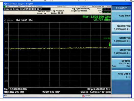
+3 dB above Out-of-band (single test signal) / 3.45 GHz Service(Ant1) / Downlink / 5G NR 40 MHz / High / Upper
