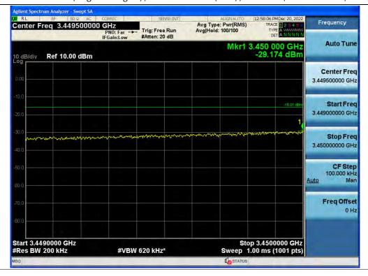
+3 dB above Out-of-band (single test signal) / 3.45 GHz Service(Ant2) / Downlink / 5G NR 20 MHz / Low / Upper
