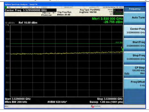
+3 dB above Out-of-band (single test signal) / 3.45 GHz Service(Ant2) / Downlink / 5G NR 20 MHz / High / Upper
