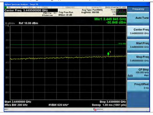
+3 dB above Out-of-band (single test signal) / 3.45 GHz Service(Ant1) / Downlink / 5G NR 60 MHz / Low / Upper
