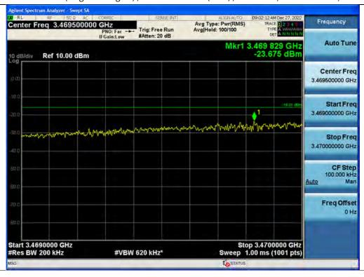
+3 dB above Out-of-band (single test signal) / 3.45 GHz Service(Ant1) / Downlink / 5G NR 60 MHz / Middle / Upper
