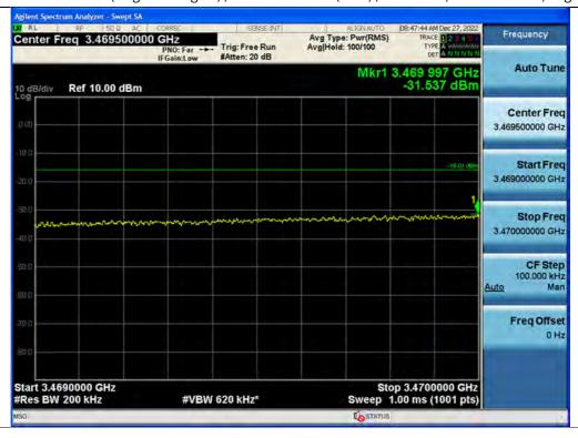
+3 dB above Out-of-band (single test signal) / 3.45 GHz Service(Ant2) / Downlink / 5G NR 80 MHz / High / Upper
