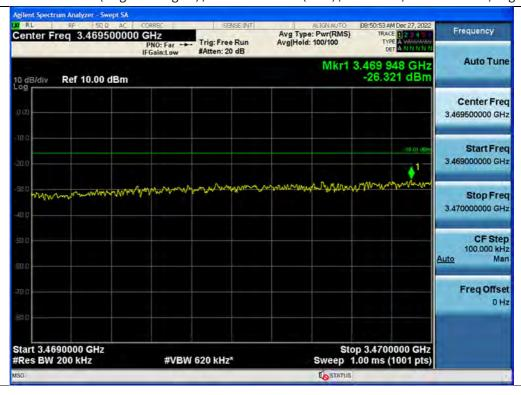
+3 dB above Out-of-band (single test signal) / 3.45 GHz Service(Ant1) / Downlink / 5G NR 80 MHz / High / Upper
