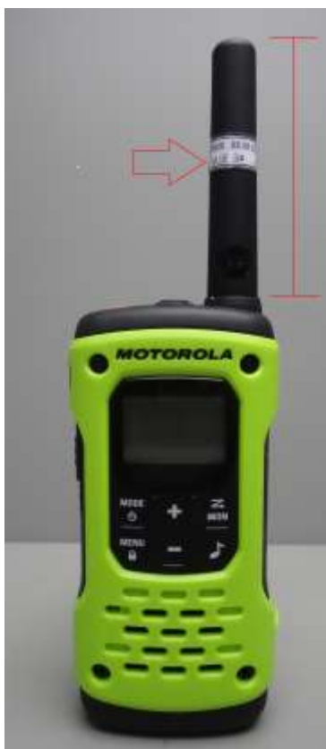
Antenna model: EAN.144F.911R (pointed with arrow)
