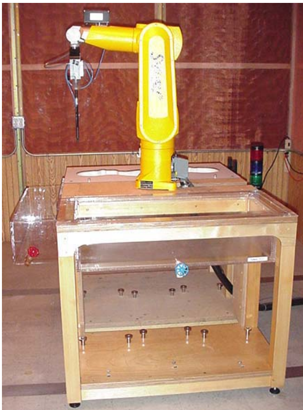
DASY4 SAR Measurement System with validation phantom
