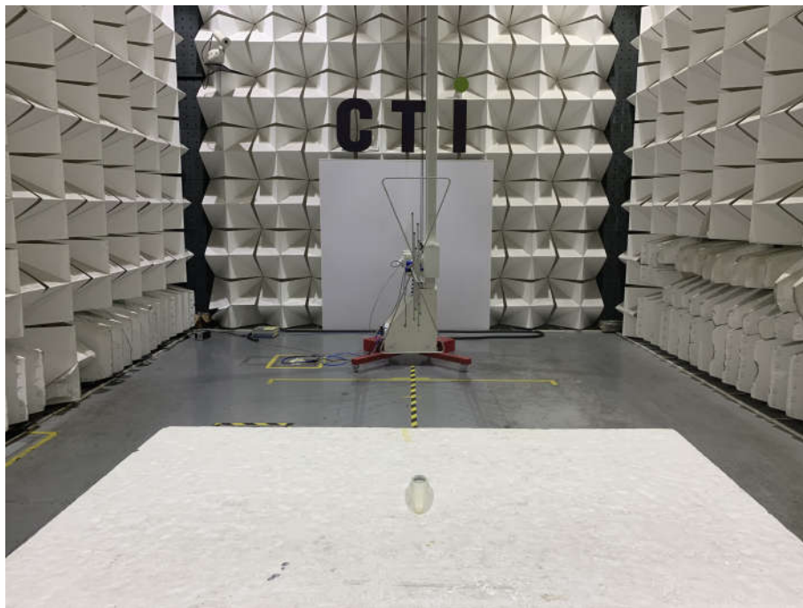
Radiated spurious emission Test Setup-1(Below 1GHz)
