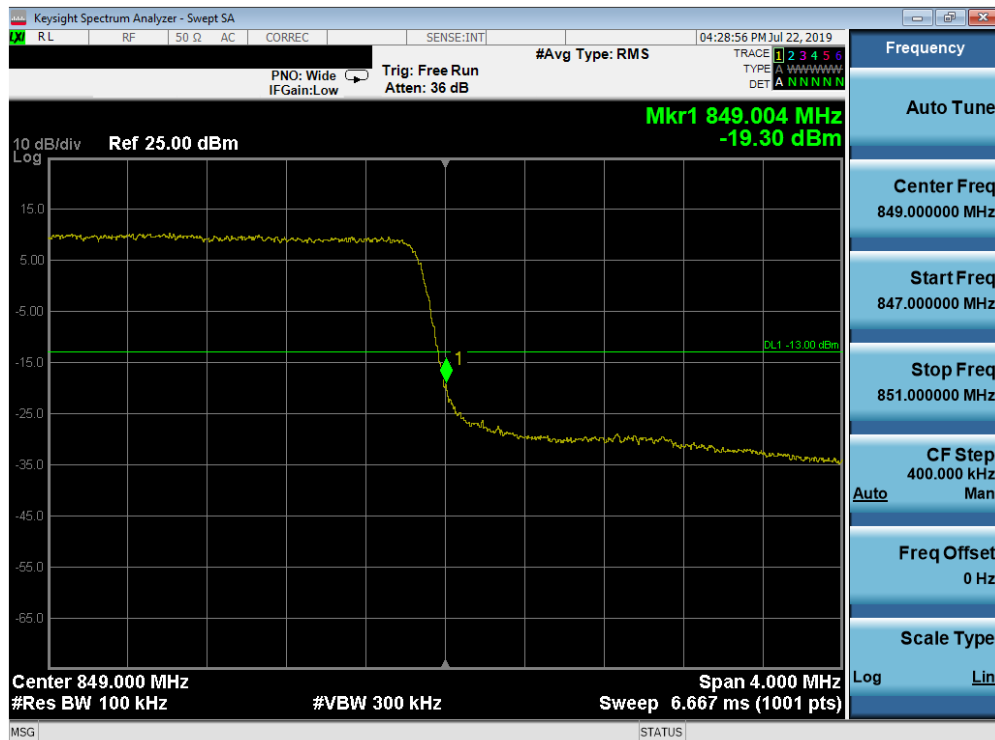
Plot 7-95. Upper Band Edge Plot (Band 5 - 3.0MHz QPSK - Full RB Configuration)
