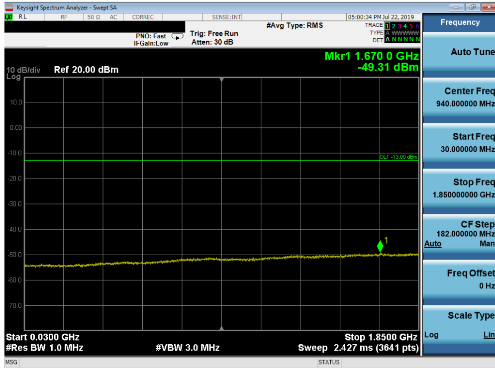
Plot 7-78. Conducted Spurious Plot (Band 2 - 10.0MHz QPSK - RB Size 1, RB Offset 0 - High Channel)
