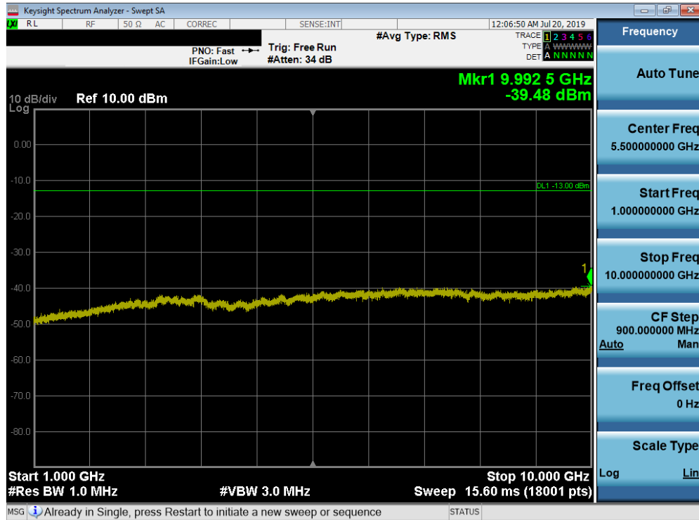
Plot 7-53. Conducted Spurious Plot (Band 12 - 10.0MHz QPSK - RB Size 1, RB Offset 0 - High Channel)
