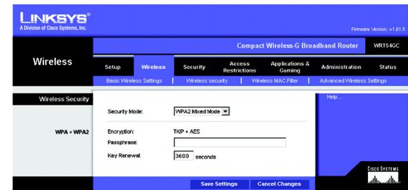
**Figure 5-18: Wireless Tab - Wireless Security (WPA2 Mixed Mode)**
