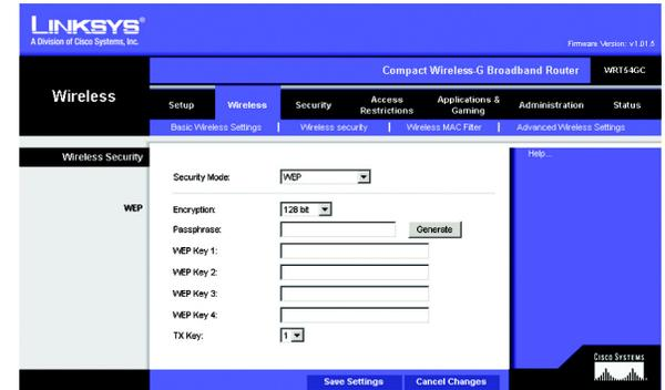
**Figure 5-15: Wireless Tab - Wireless Security (WEP)**
