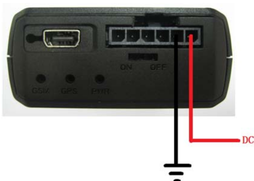
Figure 8. Typical Power Connection
