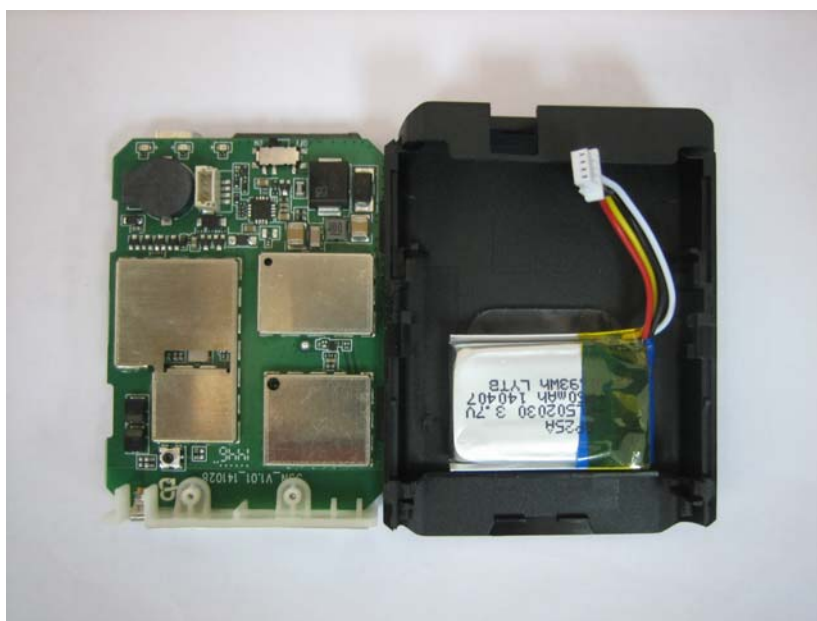
Figure 6. Backup Battery Installation
