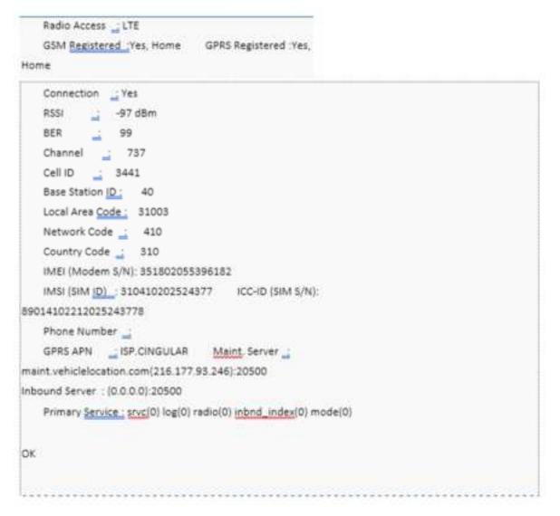
If any of the responses return Not-Acquired or Not-Registered (and the APN is correct), the wireless network operator should be contacted for further troubleshooting.
