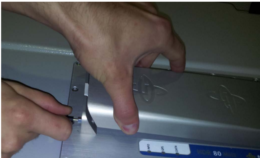
Figure 3, mounting and dismounting the battery.
