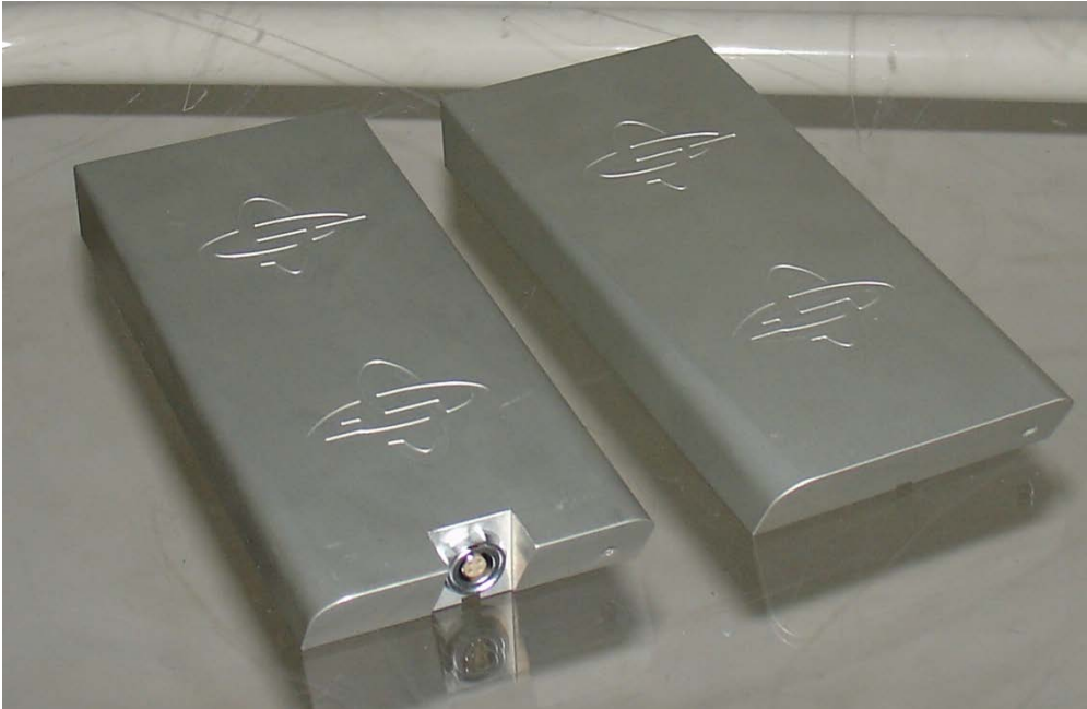
Figure 2, dummy-battery and normal LI-Ion battery.
