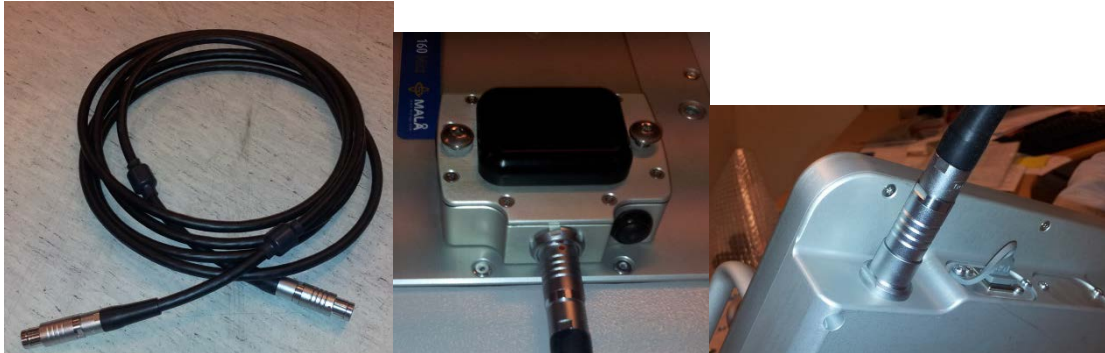
Figure 4, Left cable for communication between the monitor and HDR-unit. Cable connected to the HDR-unit and (right) cable connected to the monitor.
