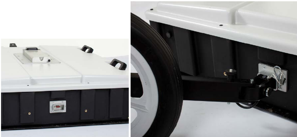
Figure 8, mounting of measruring wheels.
