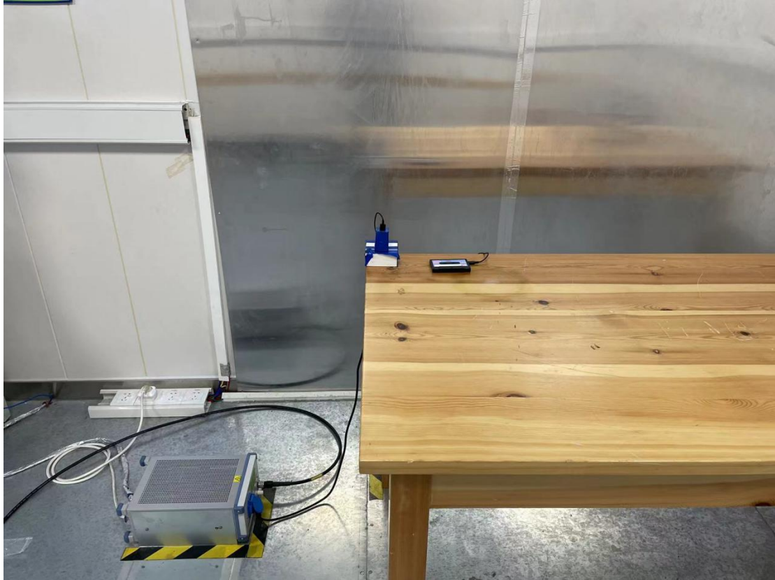
Conducted emission test setup
