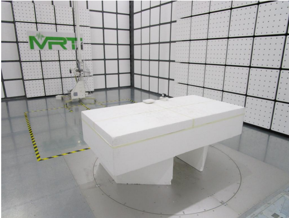
Description: Radiated Emission Test Setup for 1GHz ~ 18GHz (Test Mode 1)
