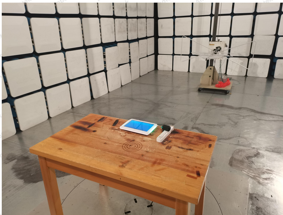
Photo of Radiation Emission Test
