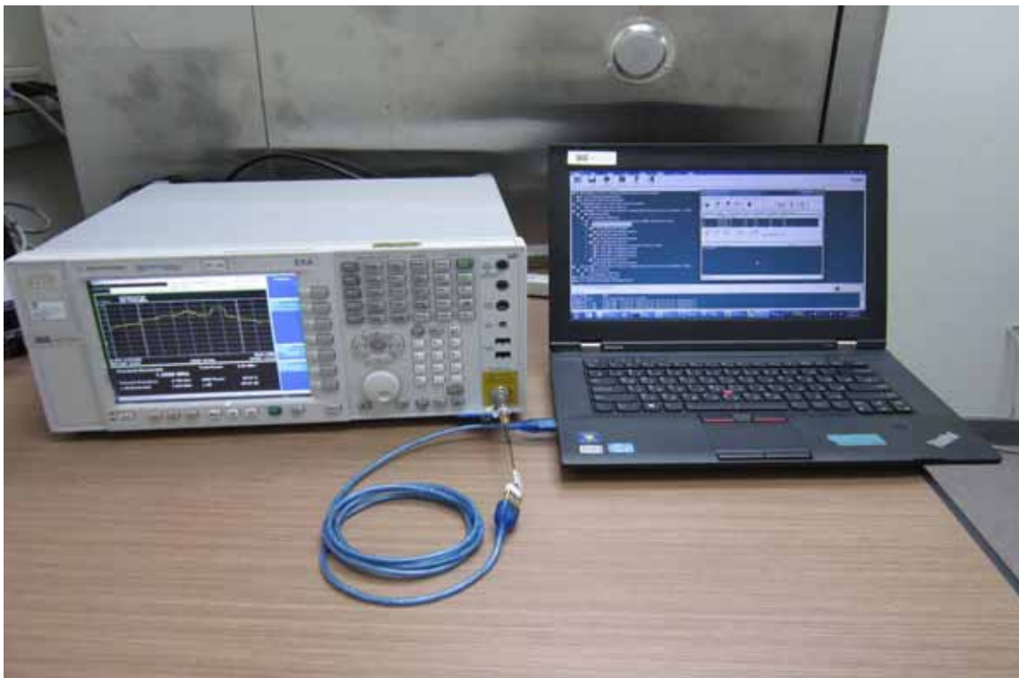
Conducted Setup Photo (Measurement at Antenna Port)
