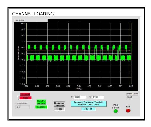
The level of traffic loading on the channel by the EUT is 33.31%.
