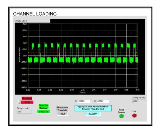
The level of traffic loading on the channel by the EUT is 33.5%.
