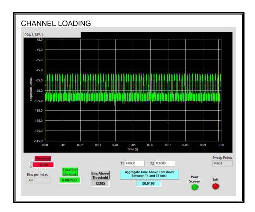
The level of traffic loading on the channel by the EUT is 30.91%.
