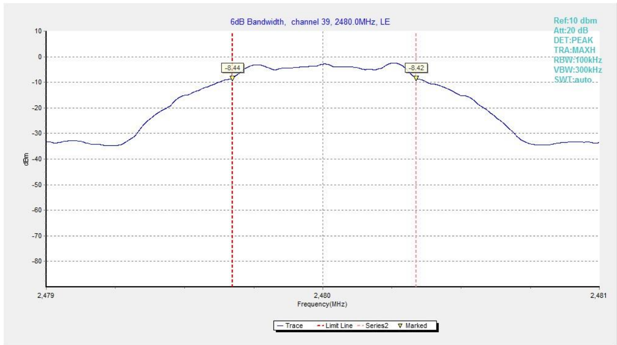
Fig.9 6dB Bandwidth (Ch 39), LE 1M
