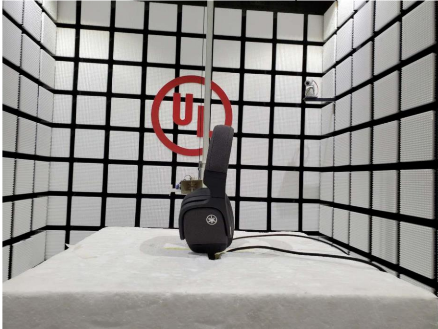
RADIATED RF MEASUREMENT SETUP (30MHz~1GHz)
