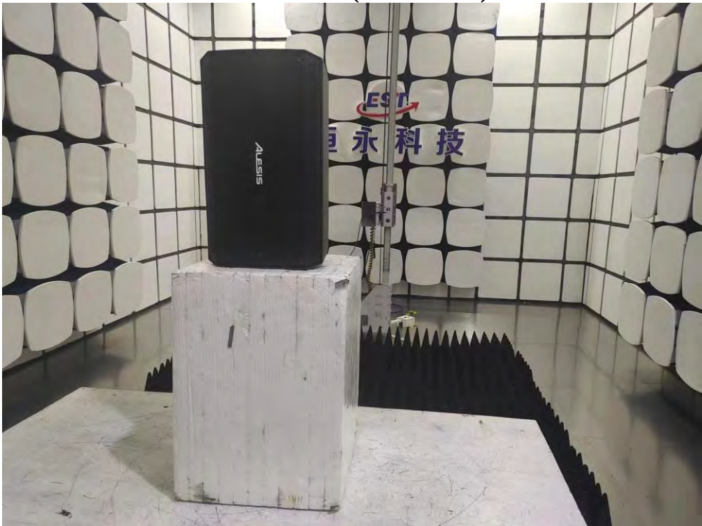
Radiated Test (Above 1GHz)
