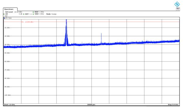
The peak above the limit is the carrier frequency. The peak at 2110 MHz corresponds to the downlink signal.
