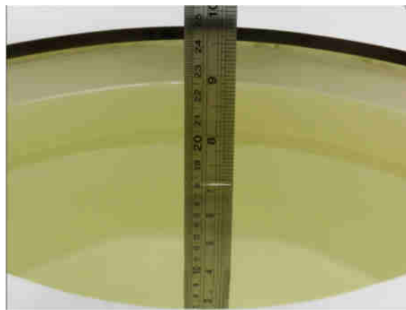
Fig 11.2 Photo of Liquid Height for Body SAR
