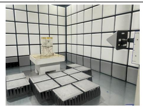
1.2 Radiated emissions set-up for frequencies above 1 GHz up to 4 GHz
