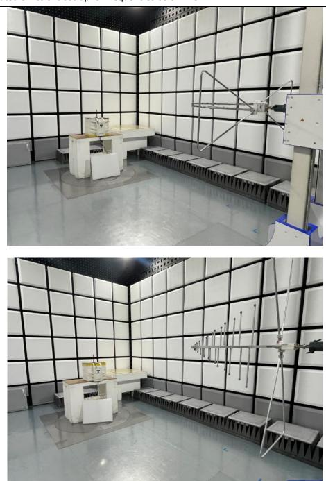
1.1 Radiated emissions set-up for frequencies below 1 GHz
