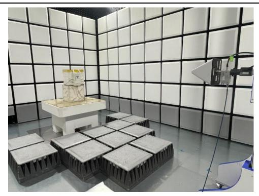
1.3 Radiated emissions set-up for frequencies above 4 GHz to 10 GHz
