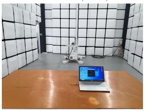
Radiated Measurement (Above 1GHz)
