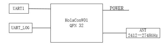
figure 1. Module System Block Diagram
