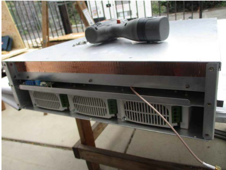
Mod #1, Copper Tape, Amplifier, View 3
