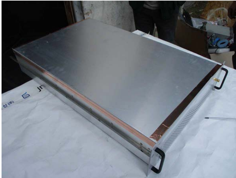
Mod #1, Copper Tape, Amplifier, View 1
