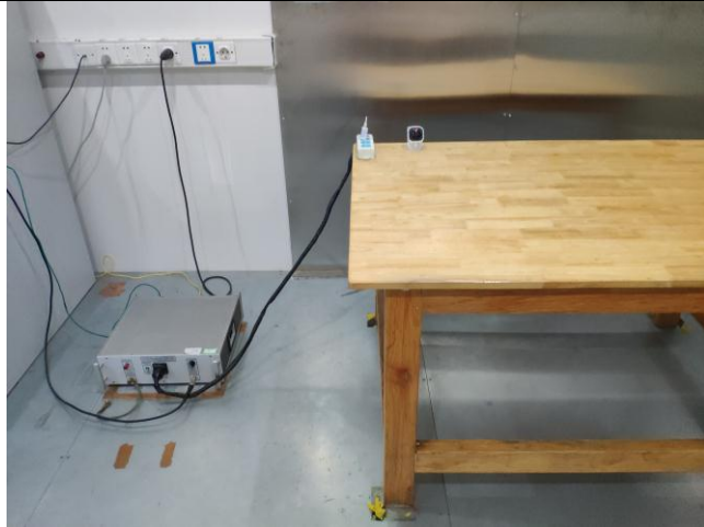
Conducted Emissions Test Setup Front View
