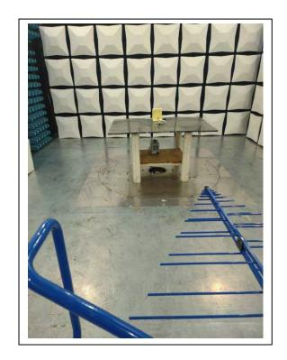
Yagi Antenna, Radiated Spurious Emission: 1 GHz to 10 GHz
