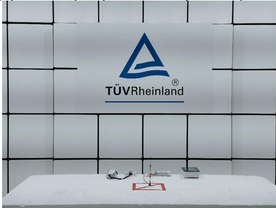
Photograph 7: Test Setup for Spurious Emissions (Front View 1)
