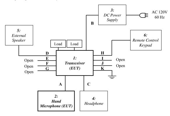
Note: The signal cable E, F, G, I and J were connected to no AE by a request from the manufacturer. 50 ohm terminals were connected to the antenna terminals (HF / VHF & UHF).
