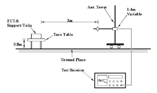
The radiated emission tests were performed in the 3-meter chamber a test site, using the setup accordance with the ANSI C63.10-2013. The specification used was the FCC Part Subpart C limits.
