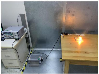
Radiated Spurious Emissions From 30MHz-1000MHz
