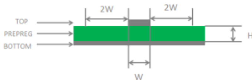
Figure 9: Microstrip Design on a 2-layer PCB
