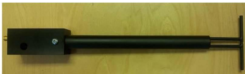
Figure 1 – MVG COMOSAR Validation Dipole
