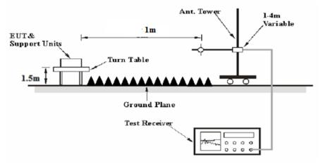
The radiated emission Below 1GHz tests were performed in the 10 meters chamber test site, above 1GHz tests were performed in the 3 meters chamber test site B, using the setup accordance with the ANSI C63.10-2013. The specification used was the FCC 15.209, and FCC 15.407 limits and RSS-247, RSS-Gen limits.
