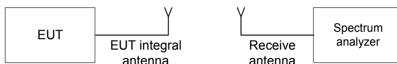
Figure 7.1.1 Setup for transmitter shut down test
