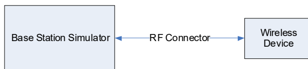
Figure 9-1 Power Measurement Setup
