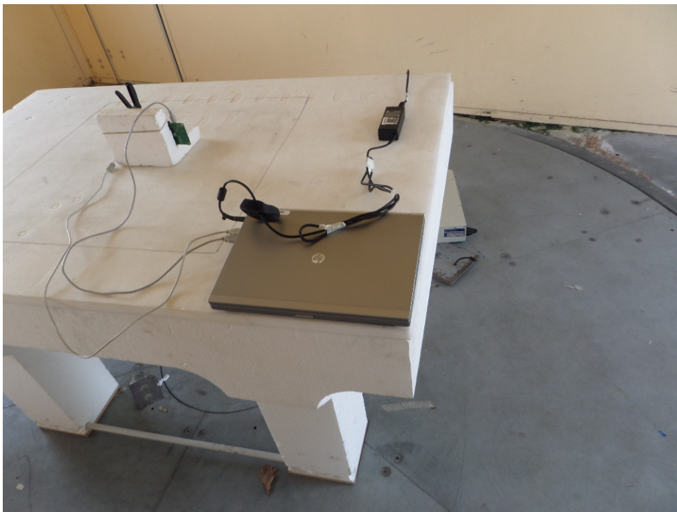
Radiated setup (open area test site)
