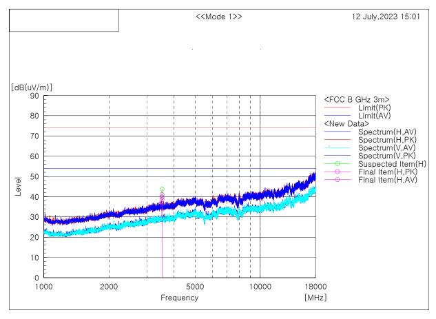
Final Result No. Frequency (P) Reading Reading Result Result Limit Limit Margin Margin Height Angle Remark c.f PK [dB] 35.3 33.0 AV [dB] 17.3 14.4 [cm] 99.8 99.8 [deg] 86.6 28.1 3515.000 3515.000
