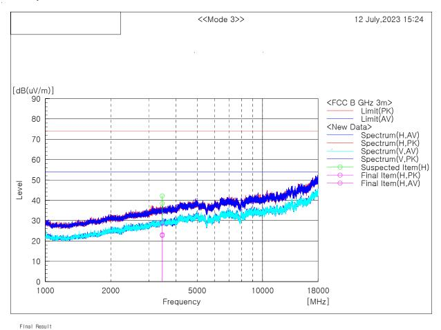
No. Frequency (P) Reading Reading Result Result Limit Limit Margin Margin Height Angle Remark c.f PK [dB] 45.1 45.0 AV [dB] 31.3 31.0 [cm] 99.8 99.8 [deg] 91.2 114.9 [MHz] 3452.000 3452.000
