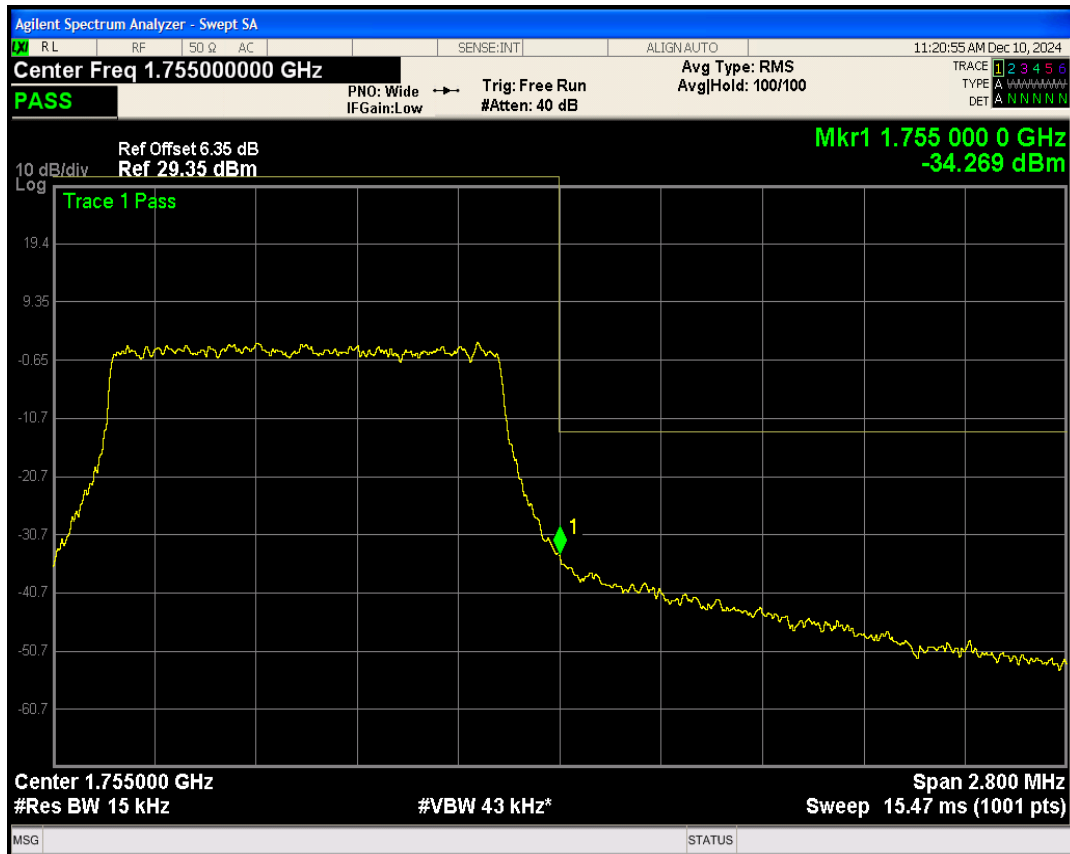
Band4 QPSK BW=3MHz Channel=19965 RB Size=15 Position=#0
