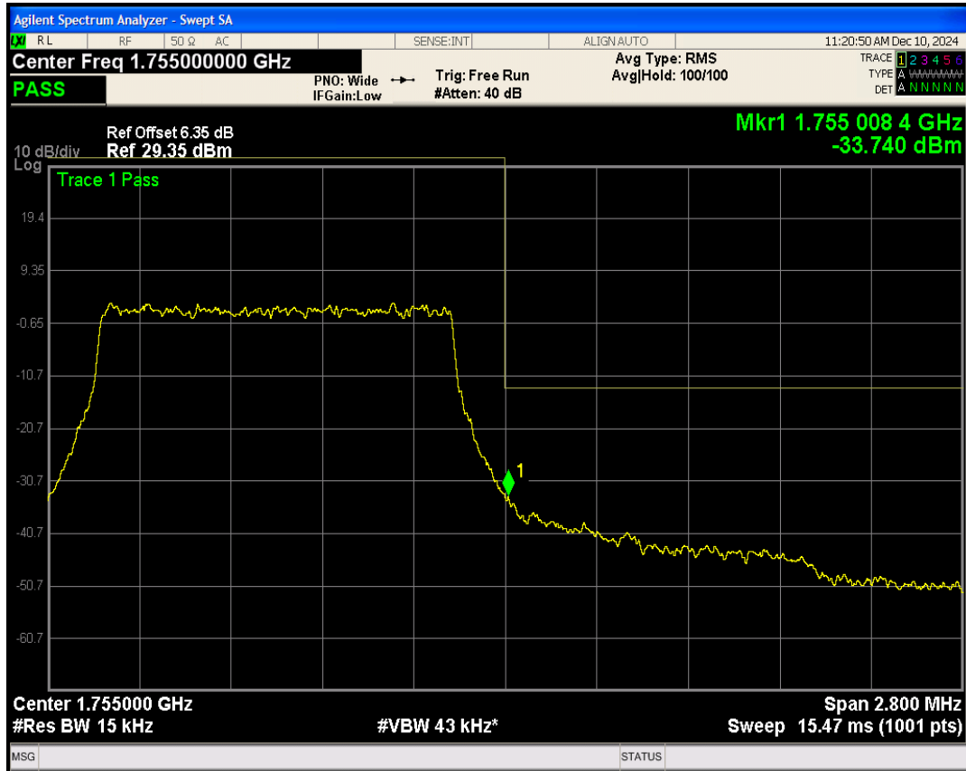
Band4 16QAM BW=1.4MHz Channel=20393 RB Size=6 Position=#0
