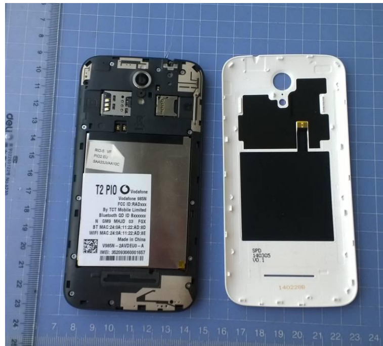
Pic A-3 Mobile phone Disassembly
