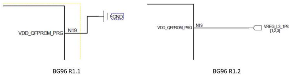
Figure 1: Schematic Designs of BG96 R1.1 and R1.2
