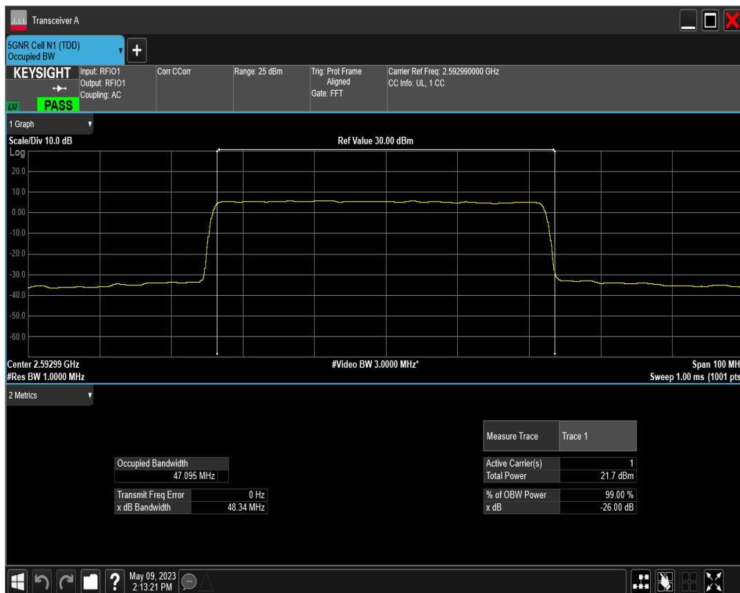
n41 SCS=30kHz CP_QPSK BW=50MHz Channel=518598 RB=133@0
