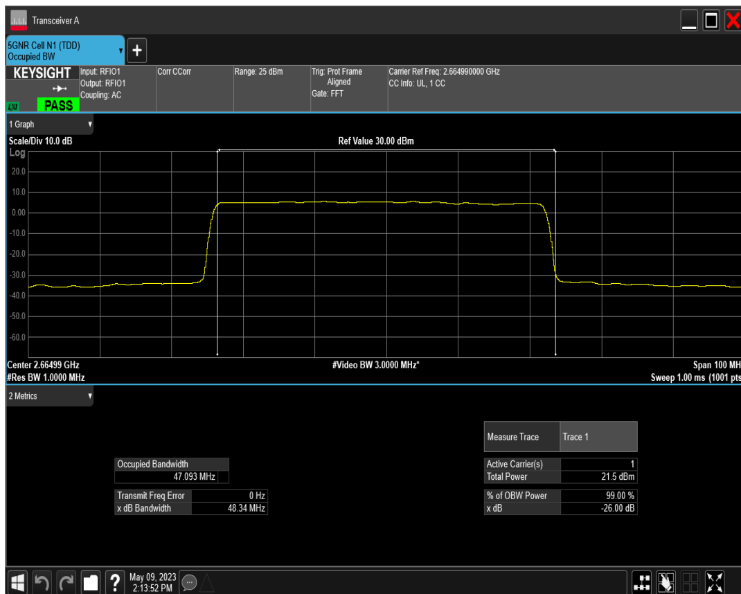
n41 SCS=30kHz CP_QPSK BW=50MHz Channel=532998 RB=133@0
