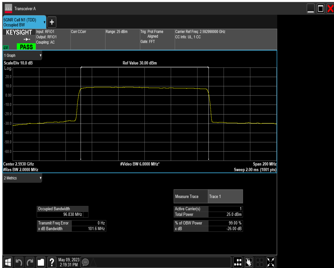
n41 SCS=30kHz DFT_QAM16 BW=100MHz Channel=518598 RB=270@0
