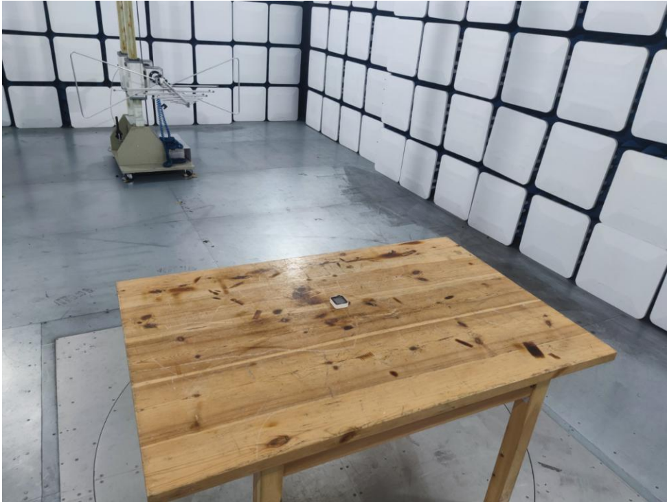
Photo of Radiation Emission Test
