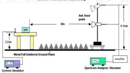
**Above 1GHz Test Setup**
