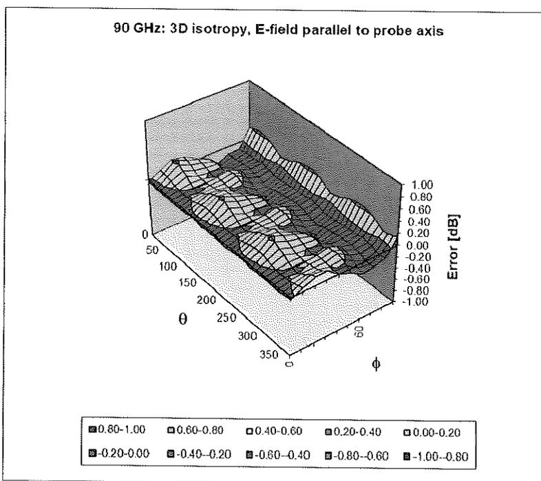
Probe isotropy for  $E_{tot}$ : probe rotated  $\phi = 0^\circ$  to  $360^\circ$ , tilted from field propagation direction  $\vec{k}$
