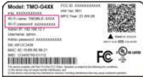
The QR code on the label provides easy set up when the T-Mobile Internet mobile app is installed.
