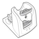
4. Insert the MC3330U device into the MC32N0 cradle.
