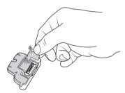
3. Insert the adapter into the MC32N0 cradle and adhere it to the bottom of the cradle.
