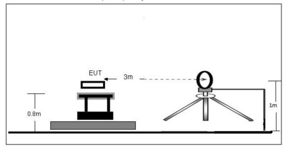
(B) Radiated Emission Test-Up Frequency 30MHz~1GHz
