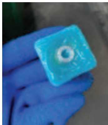
Figure: DynaLogger installation with glue fixation
