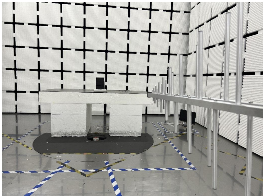
Radiation Emission Test Setup (30MHz to 1GHz)
