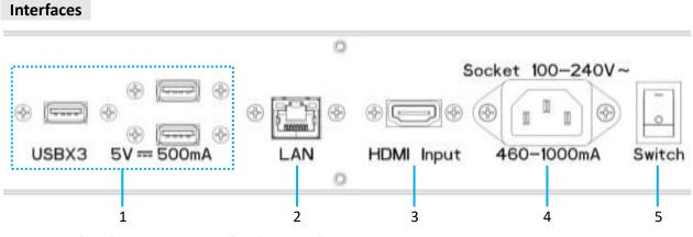
1. USB interface \* 3, 2. RJ45 interface(Ethernet), 3. HDMI input, 4. Socket, 5. Switch, Note: Please pull out the power plug before installing or disassembling the unit!
